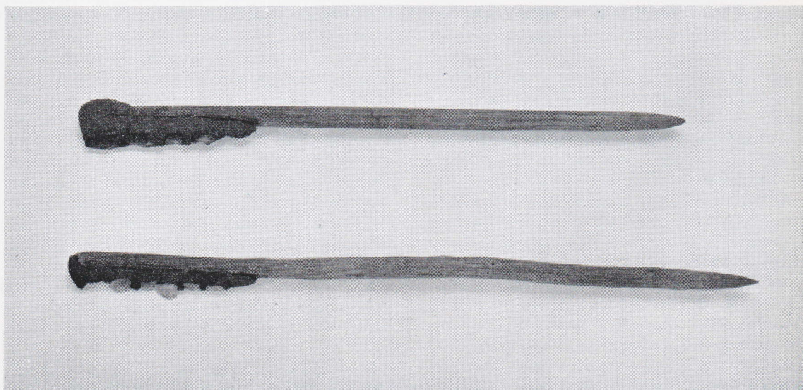
4. Two modern primitive saws from Western Australia; they are made from stone and glass flakes set in gum
