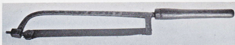
38. 18th century Swedish hacksaw. Another example, the blade much worn by repeated sharpening
