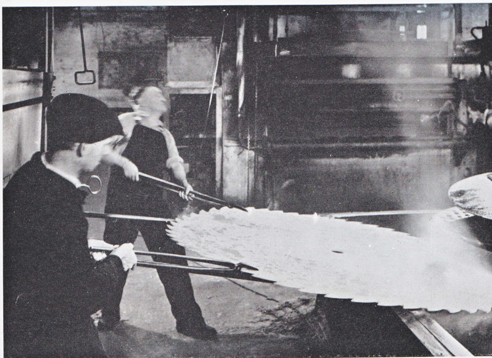
73. Hardening the heated blade by quenching in oil. A 72-inch diameter solid tooth saw at red heat is quenched
