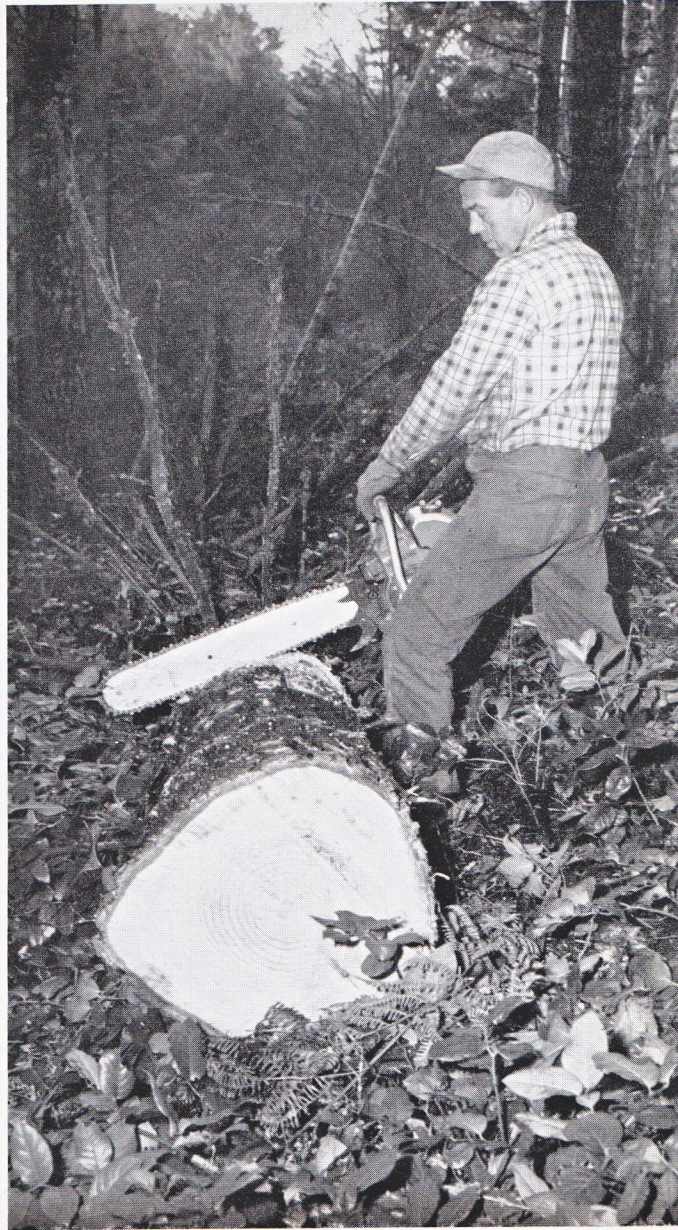
94. Felling in the forest by power-operated saw chain
